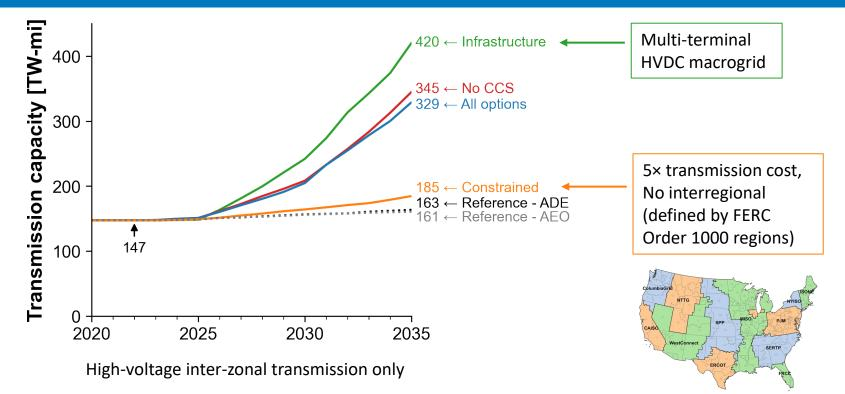
These large transmission buildouts enable access to high-quality, low-cost resources, and only contribute ≤10% to overall system cost
