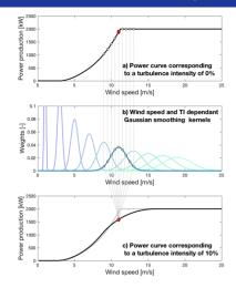
**Figure:** Effect of turbulence near rated wind speed. Figure from Saint-Drenan et al. 2020 DOI: 10.1016/j.renene.2020.04.123
