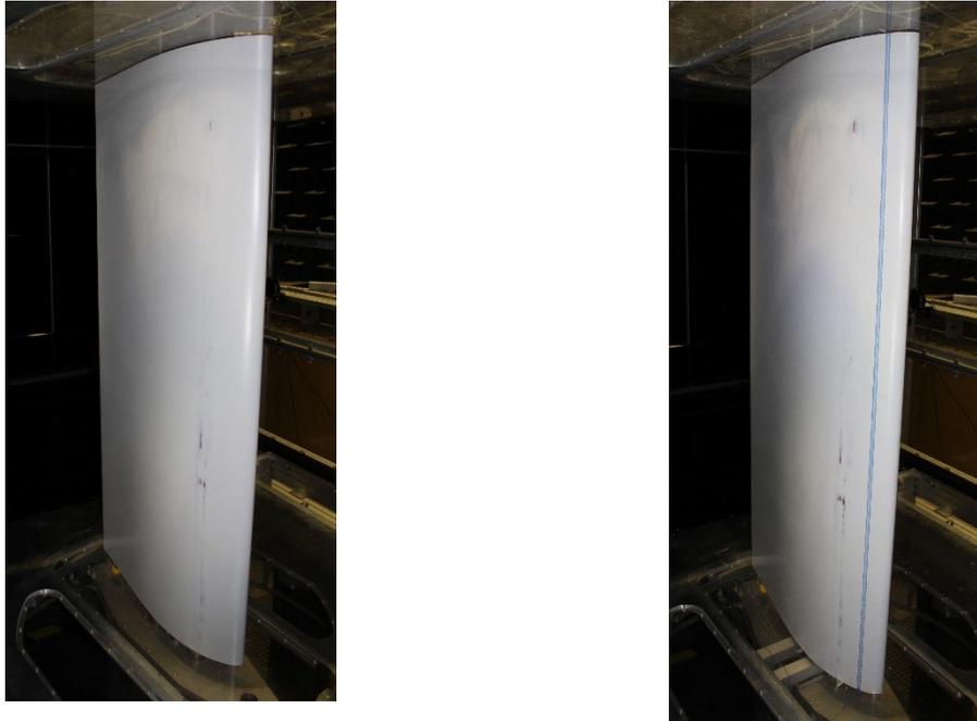
**Figure 11: FFA-W3-211 in the PLCT clean (left) and zigzag-tape (right).**
