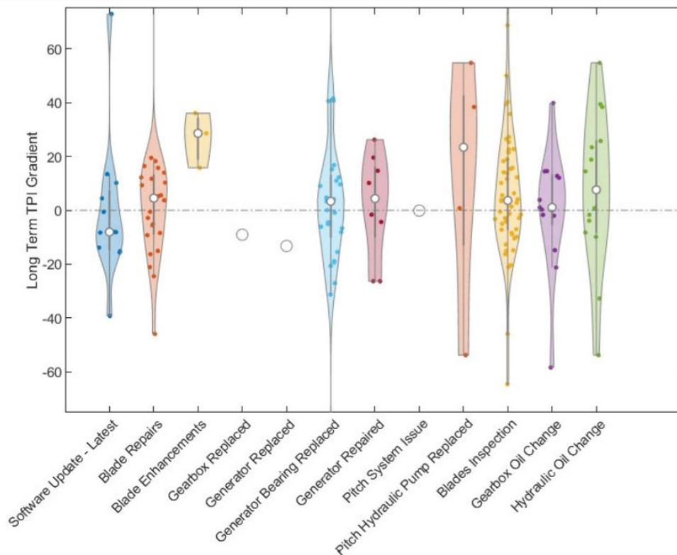
**Figure 8** Violin plots of TPI (Turbine Performance Integral) plotted in connection to each maintenance activity. Illustration from (Malik & Bak, 2024).
