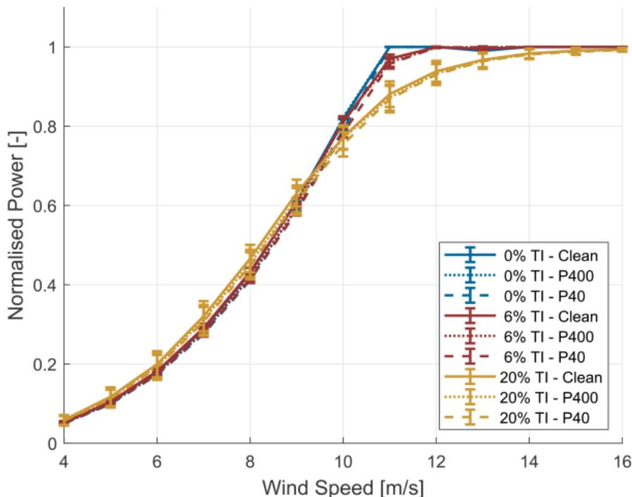
Figure 6. Normalized power for a MW wind turbine as a function of wind speed. The performance for 0%, 6% and 20% turbulence intensity is shown, where also three different levels of aerodynamic performance are shown: A clean blade, a blade with a lightly eroded leading edge corresponding to a sand roughness of P400 and a blade with a heavily eroded leading edge corresponding to a sand roughness of P40. Illustration from (Malik & Bak, 2025A).
