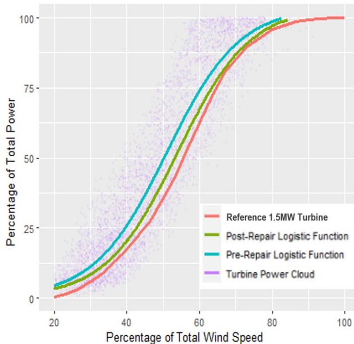
**Figure 2. Regression power curves produced for observations before and after each turbine repair date.**
