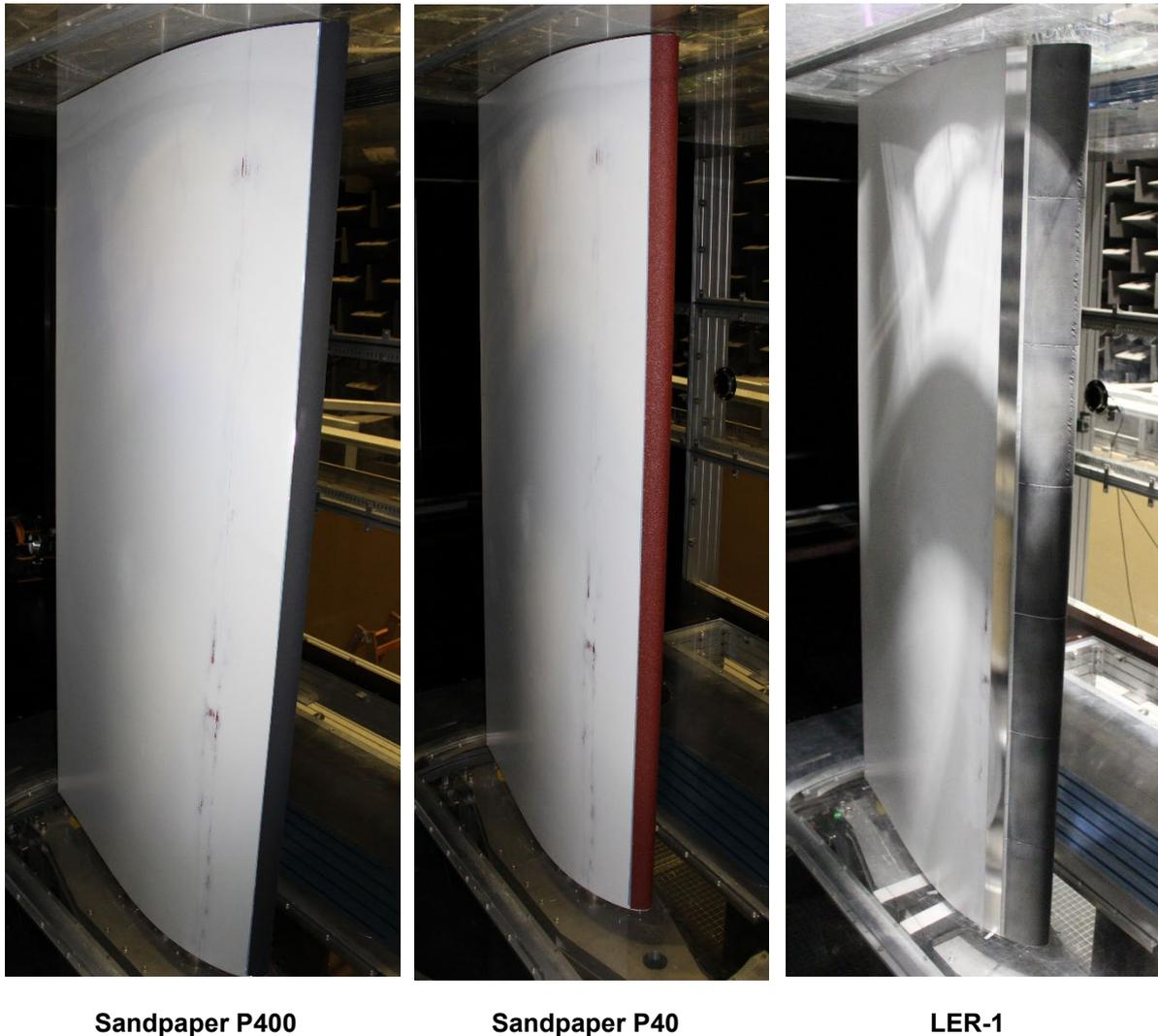
**Figure 12: FFA-W3-211 in the PLCT with different LEE applied**
