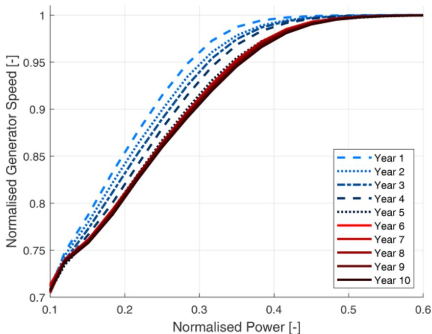
**Figure 7 Normalized generator speed as a function of normalized power for each year for a wind turbine. Illustration from (Malik & Bak, 2024).**
