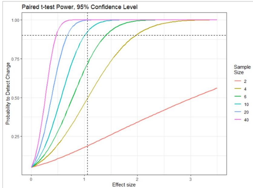
**Figure 5. Required turbine pair sample size as a function of the probability to detect an increase in the relative power output of a set of turbine pair samples, modeled using a one-sample t-test of differences.**
