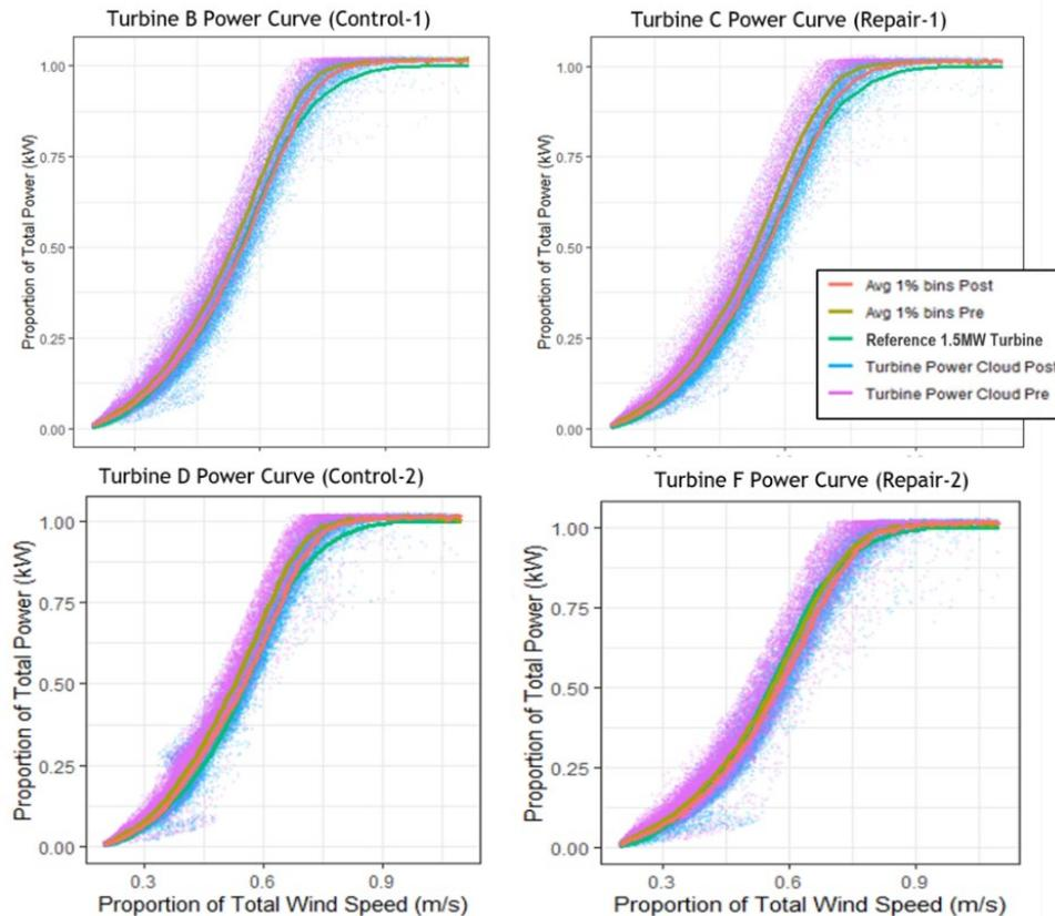
**Figure 3. Comparison of power from turbine pairs. Power normalized by rated power and wind speed normalized by the rated wind speed.**
