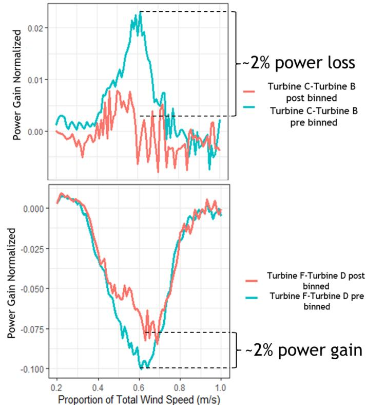
**Figure 4. Relative power difference between turbine pairs C and B (top) and D and F (bottom).**
