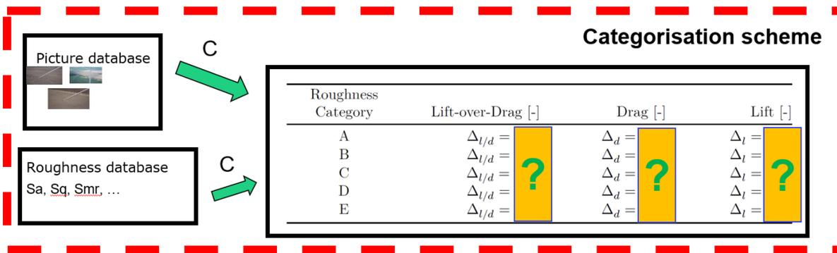
Figure 13: Draft of the LERCat categorization scheme that links blade inspections with a sectional aerodynamic loss.
