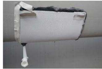
2: Mould for silicone imprint on the blade
