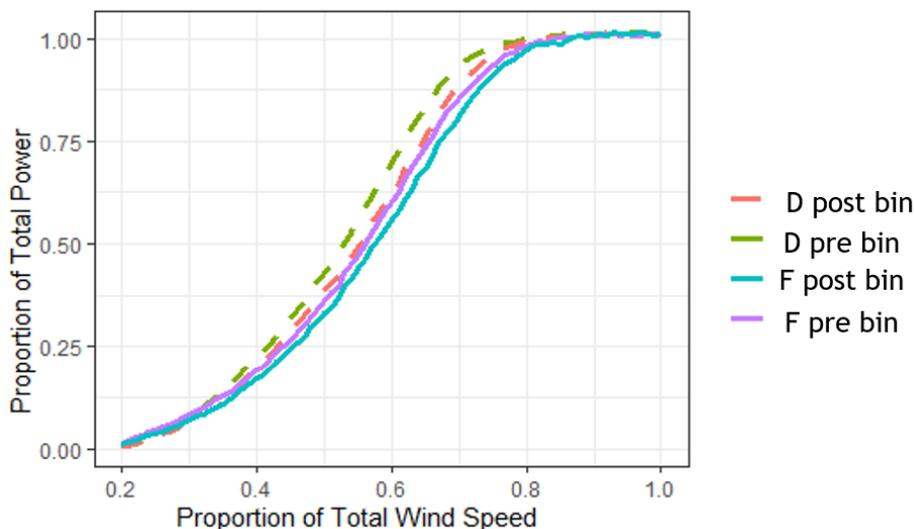
Figure 1. Average wind speed binned power curves for turbines D and F.
