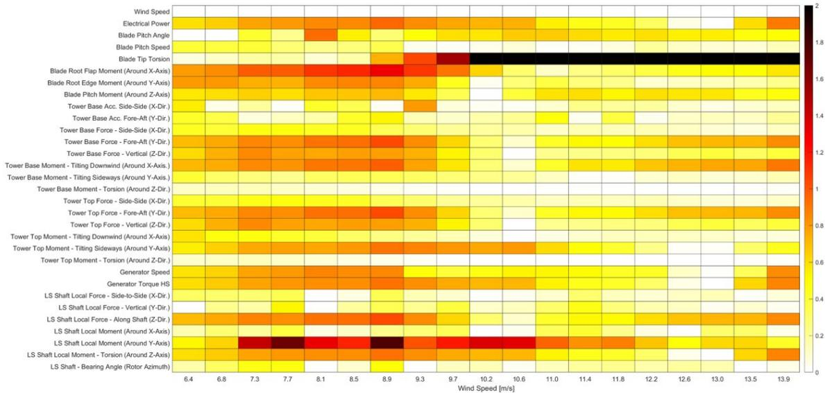
**Figure 9** Heat map of the difference in performance for rough (P40) versus clean conditions as a function of wind speed for multiple sensors at a turbulence intensity of 12 %. Illustration from (Malik & Bak, 2025B).
