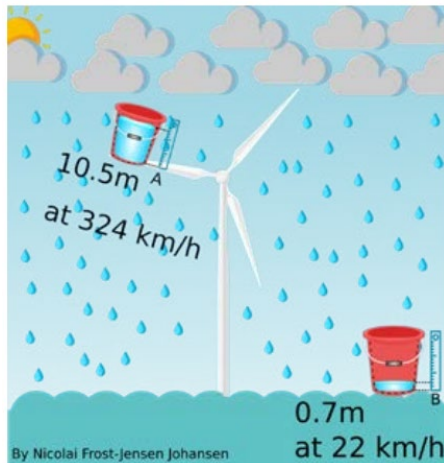
Figure 5. Illustration of annual rain amount hitting 1 cm 2 on the tip of a blade, the closing velocity between the blade and the falling rain droplet being 324 km/h (bucket A), versus rain on the ground hitting 1 cm 2 with a closing velocity of 22 km/h between the land surface and the falling rain droplet (bucket B). From Hasager et al. 2021.
