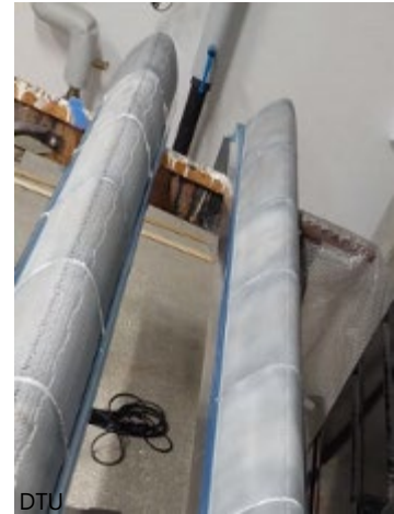
Eroded leading edge models from DTU LERCat project.
