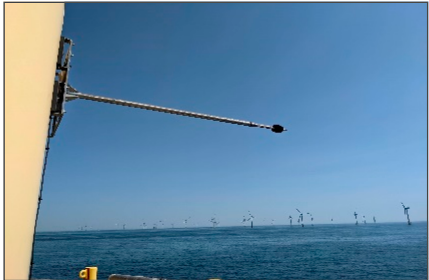
Figure 3: Microphone test set-up at Rentel offshore wind farm. (Source: Sirris.)
