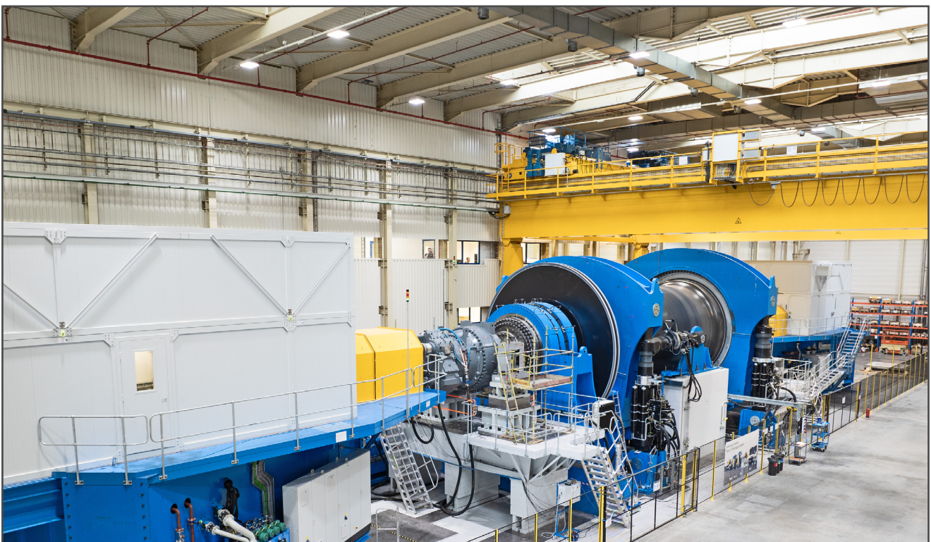
Figure 4: ZF Power validation test bench. (Source: ZF Power.)
