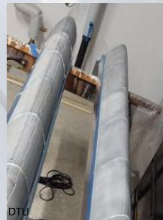
Eroded leading edge models from DTU LERCat project.
